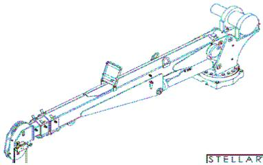
**STELLAR MODEL 7621W Crane** -- 6000 lb Lift Capacity @ 6 ft Mounted on rear corner of flatbed body with wireless remote control and auxillary cord. 11ft to 20ft power extendable boom. Includes 15 gallon hydraulic reservoir w/filter, 20ft pressure and suction hose, fittings and 17 gallons of hydraulic fluid.
