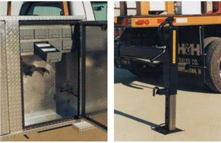
Equipto® pull out drawer unit. Outrigger shown in down position.
