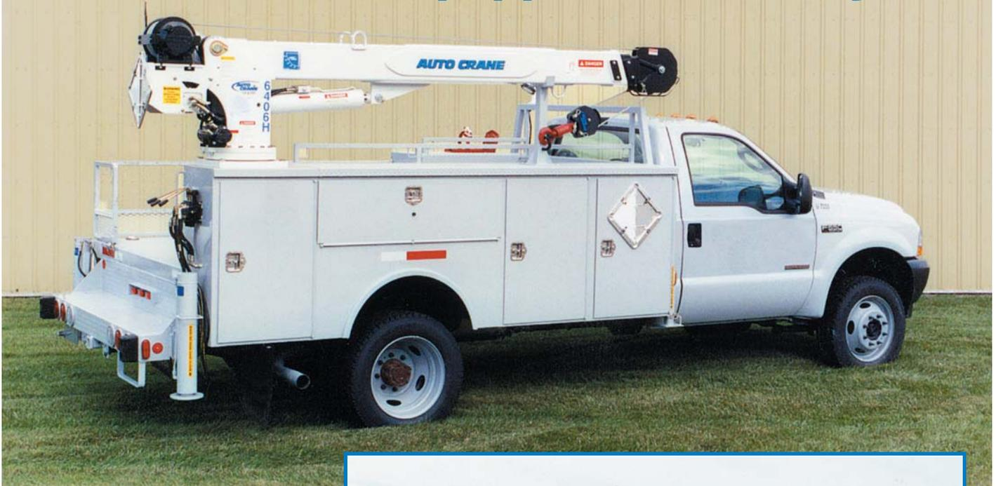
**Model 96-132KM with hydraulic outriggers and 6406H crane.**
