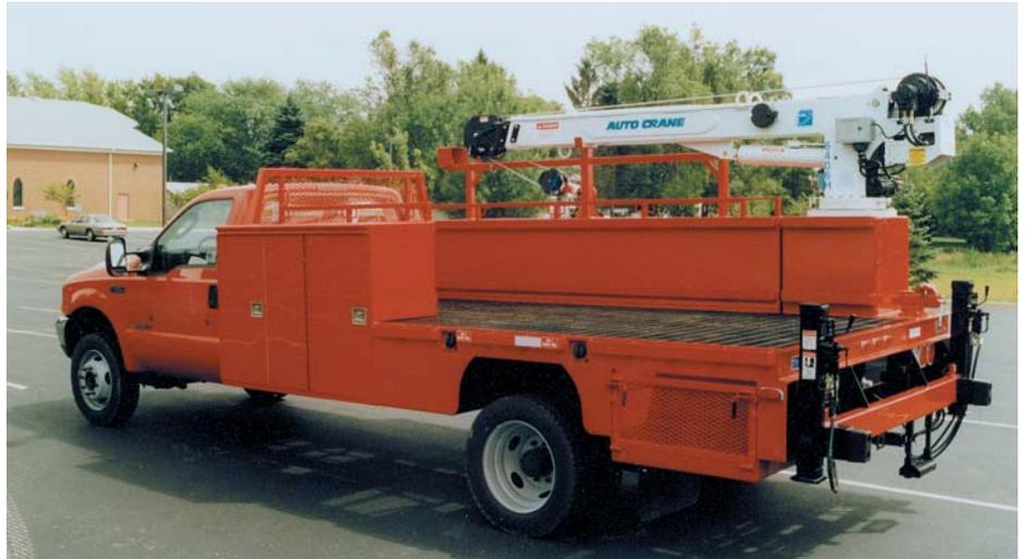
**Model 96-169KM with front mounted, street-side tool boxes and hydraulic outriggers (above).**
