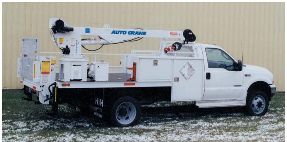
Model 96-144EM with 1500 lb. capacity lift gate.
