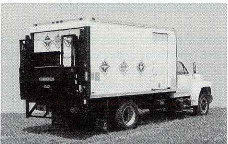
Fully enclosed, all aluminum cube van bodies are available for weather protection and security.
