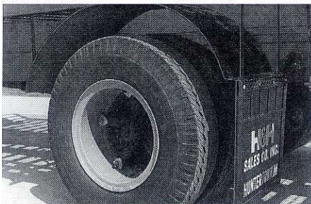
Rear wheel fenders prevent tires from throwing road debris through the grated floor.
